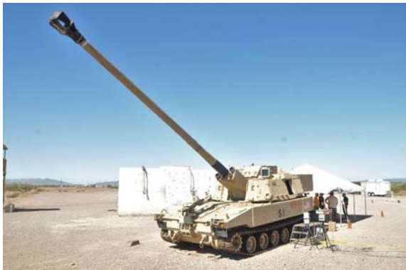
M1299 ERCA. Note the extended length of the barrel. Source: Defense News
